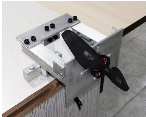
Figure 4. Testing device for the determination of propeller lifting force.
