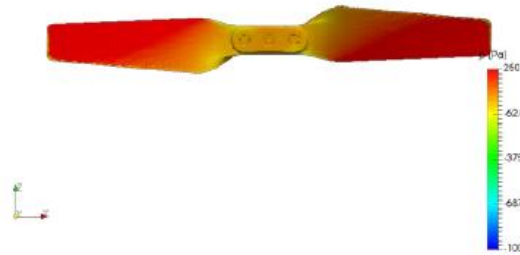
Figure 9. The pressure distribution at the bottom surface of the blade for the original propeller
